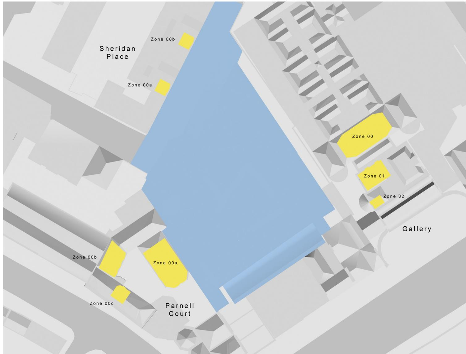
**Figure 5.12.1:** Location of sample windows assessed as part of this sunlight access impact analysis (Shown in yellow)
